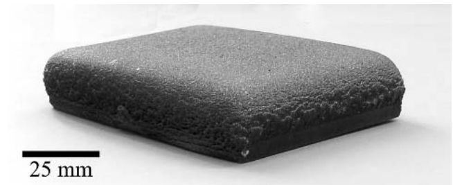
Fig. 4 Optical micrograph of 20,000 \mu\text{m} thick SHS7170 wire-arc coating deposited onto a 0.635 cm thick 1018 plain carbon steel
